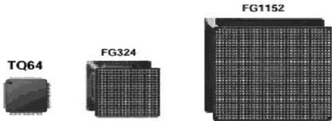
Fig.1.3: Examples of FPGA Packages
