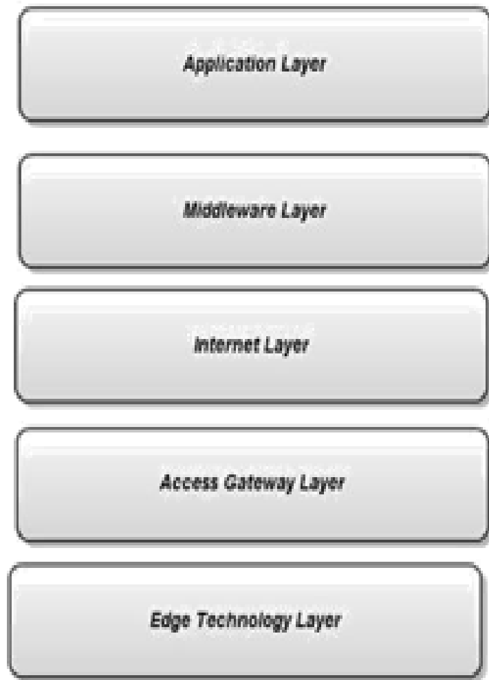
Figure 4.3. Layered architecture of the Internet of Things (IoT)
