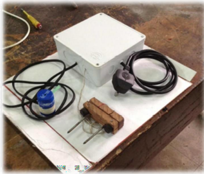
Figure 2.1 Auto irrigation system
