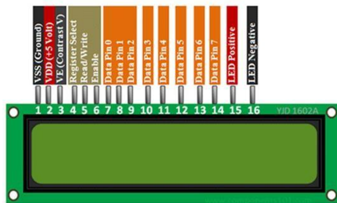
Figure 4.7 - 16x2 LCD (Liquid crystal display)
