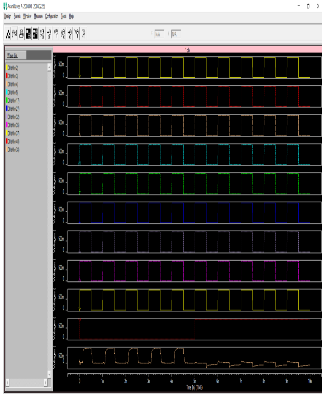
Figure 5.3 Simulation output of a CLB 32nm with P-HALF SLEEP.
