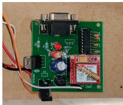
Fig: 4.17: SIM800L on Circuit Board.
