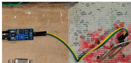
Fig: 4.13: Soil sensor on Circuit Board.
