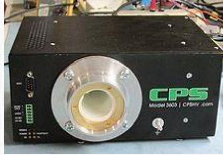
Fig 4.19 High-voltage power supply
