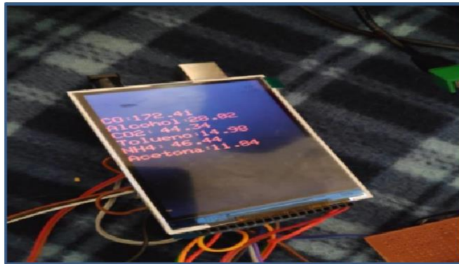
Values of gas sensors on display module
