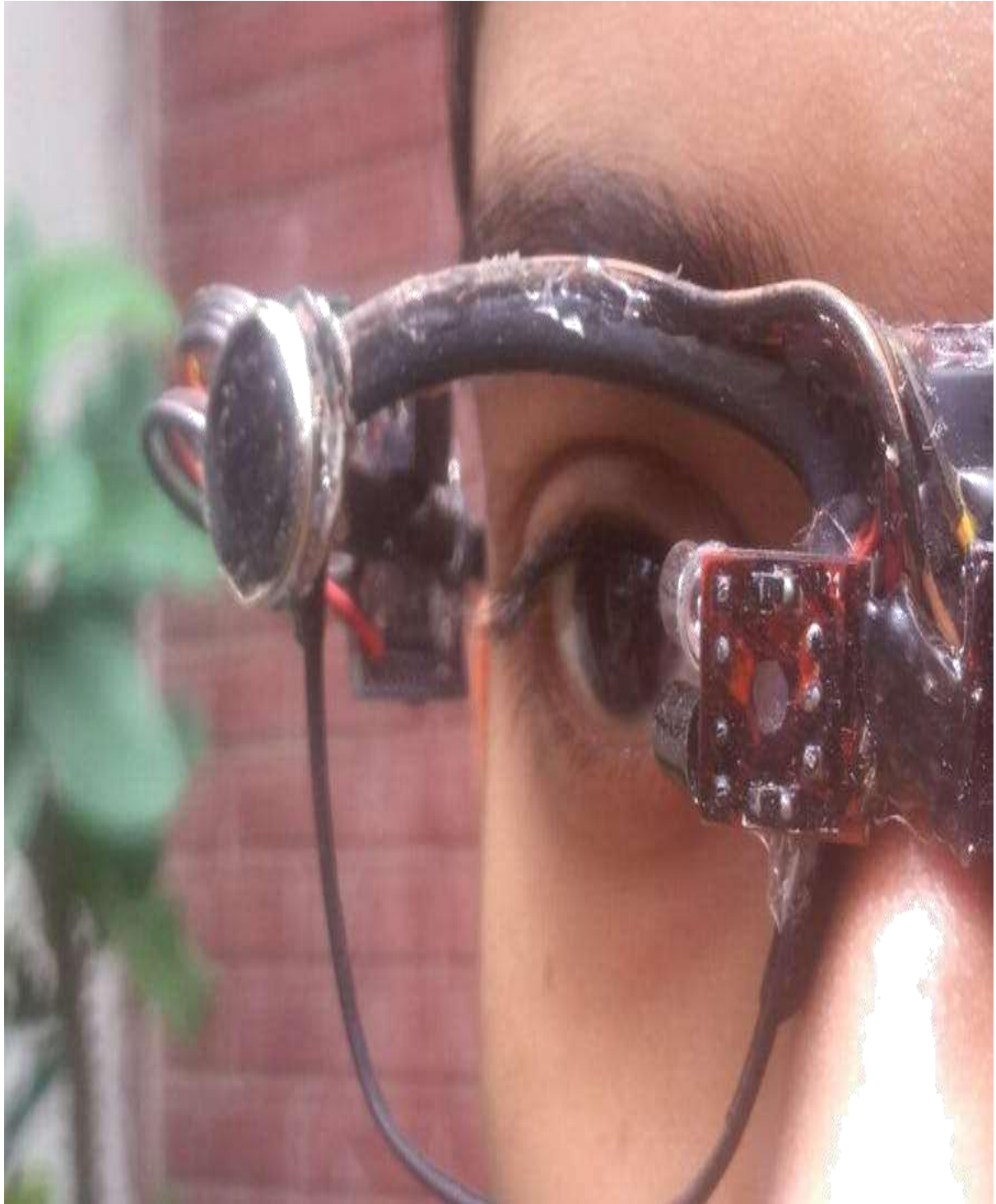
Fig 4.8 IR SENSOR IN GOOGLES
