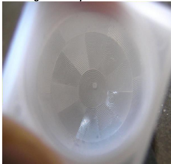
Fig 4.10 This macro shot shows the different Fresnel lenses in each facet!
