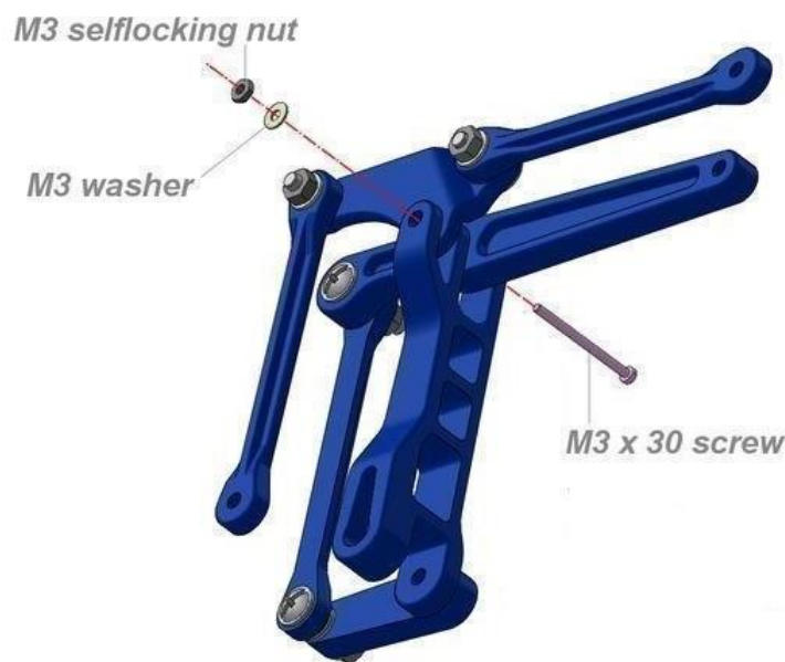
Figure 6.1 robotic arm assemble (step 1)
