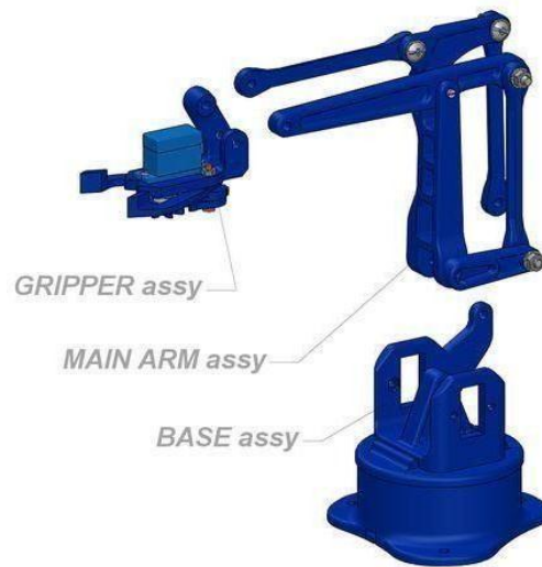
Figure 6.4 robotic arm assemble
