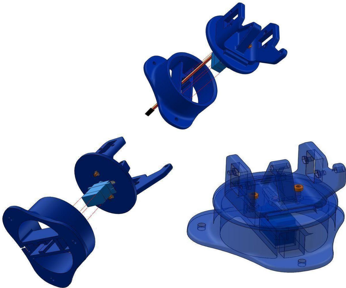
Figure 6.2 robotic arm assemble (step 2)
