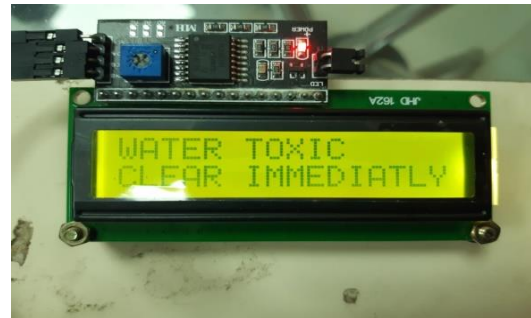
Fig:5.12 : Alert Messages on 16x2 LCD display
