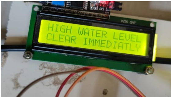
Fig:5.12 : Alert Messages on 16x2 LCD display
