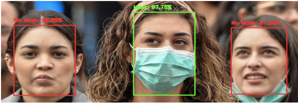
Fig 3.1 :human face with and without mask detection
