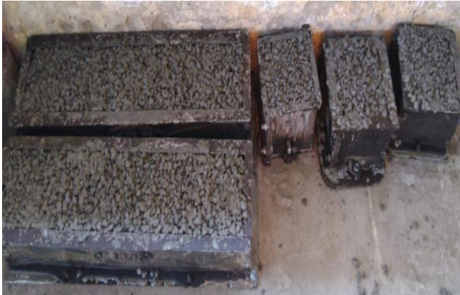
Fig 4.5 Refers to the moulds of beam and prism
