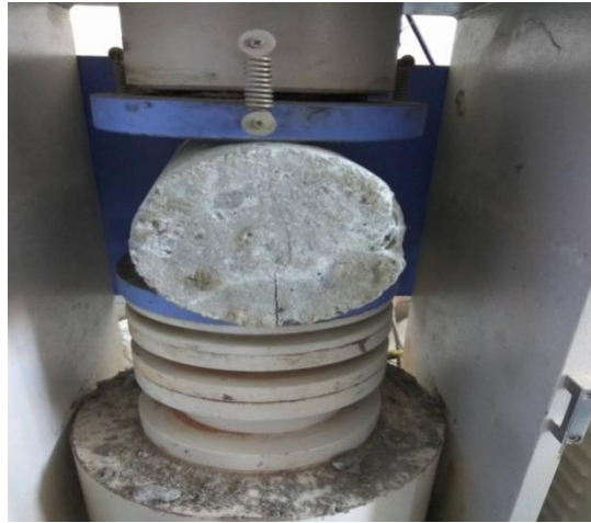
Fig: 5.3 Tensile Strength Test of Concrete
