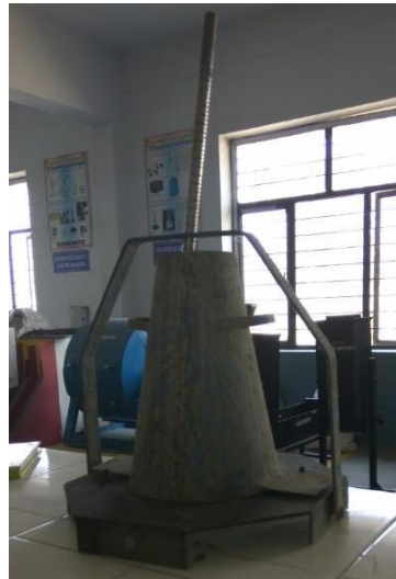
Fig:5.1 Slump Specimen
