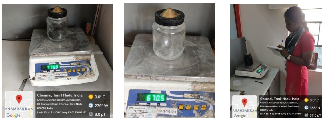
Fig 4.14: Specific gravity of Reed plant ash
