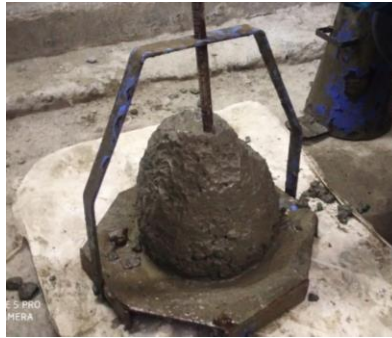
Fig 4.16: Slump test for concrete mix
