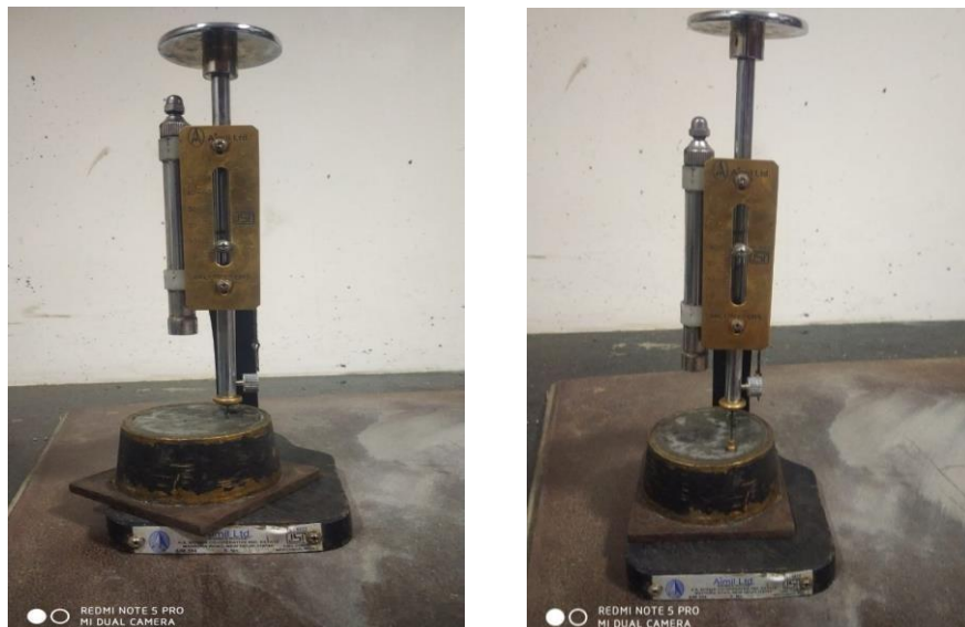
Fig 4.9: Initial and final setting time of cement
