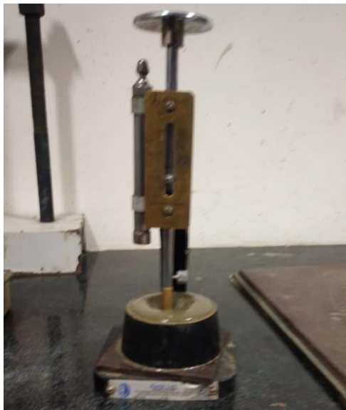
Fig 4.8: Consistency of cement test
