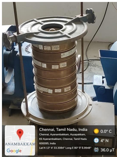
Fig 4.11: Finding Fineness modulus of fine aggregate
