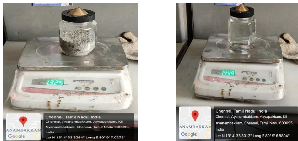
Fig 4.10: Specific gravity test for fine aggregate
