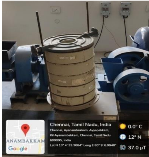
Fig 4.13: Fineness modulus test for coarse aggregate
