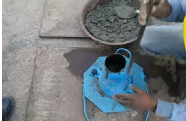
Fig 6.1 slump cone test
