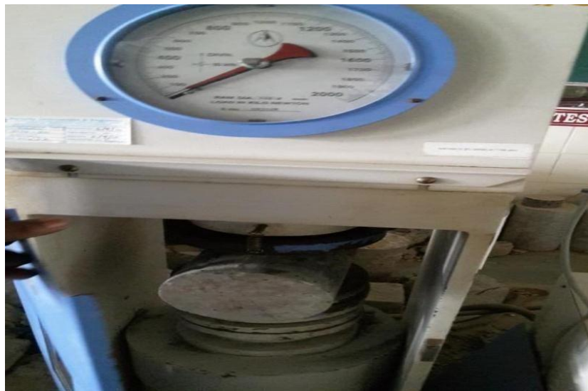
Fig 3.11 Split Tensile Testing
