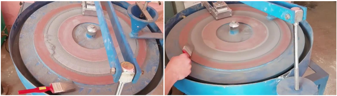
Fig: 5.4: Abrasion test done on concrete tile
