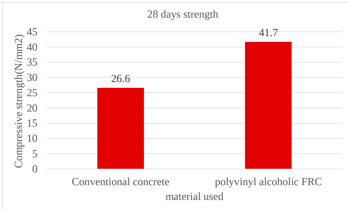
FIGURE 5.2 Compressive Strength for 28 days
