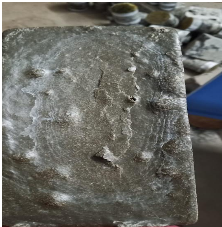
Fig. 5.2 Failure of the specimen at the maximum load
