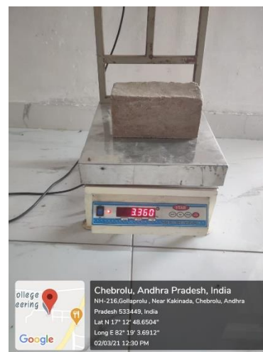
Fig. 5.6 weight of cement plastic brick (1:1:3) Fig.5.7 weight of plastic brick (1:4)
