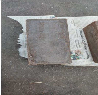
Fig 4.2 MIX PROPORTIONS OF BRICKS (1:3)
