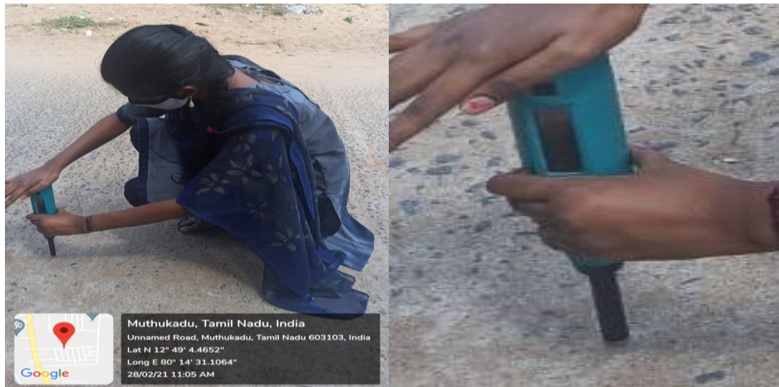
Fig:4.19 : Performing Rebound Hammer test
