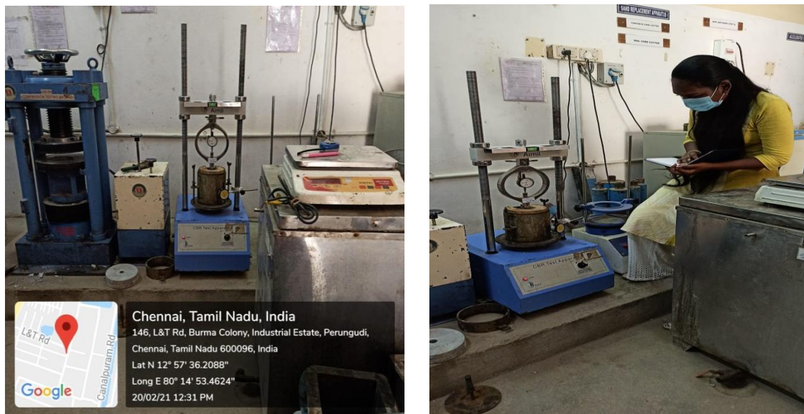
Fig:4.15 :California Bearing Ratio testing apparatus
