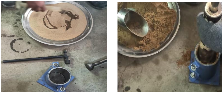
Fig:4.13 :Proctor standard density testing apparatus
