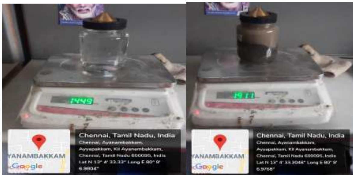
Fig:4.8 : Specific Gravity Test For Fine Aggregate
