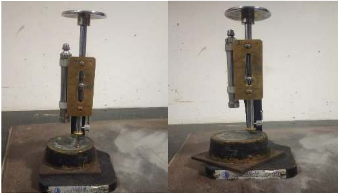
Fig:4.7 : Consistency of Cement
