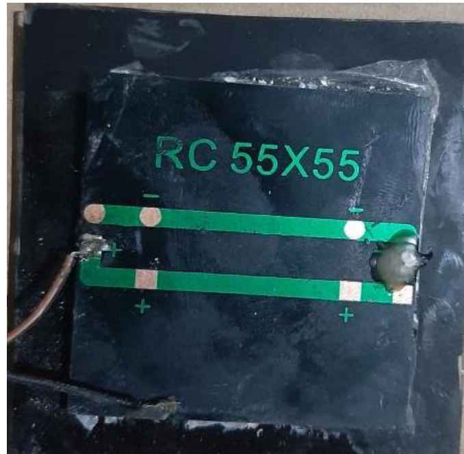
Fig 5.1.1: Heating panel (5v)
