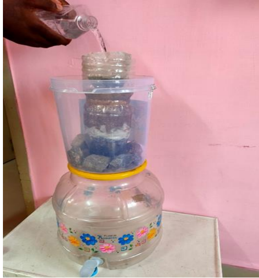
Fig: 4.21: Pouring of raw water for filtration
