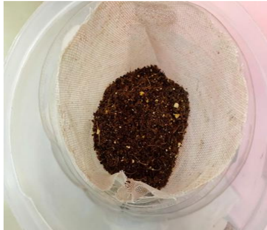
Fig: 4.20: Banana peel powder in filter media
