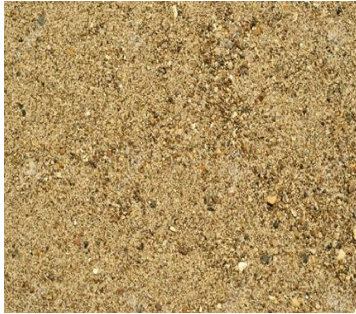
Fig: 4.14: Sand used for filtration
