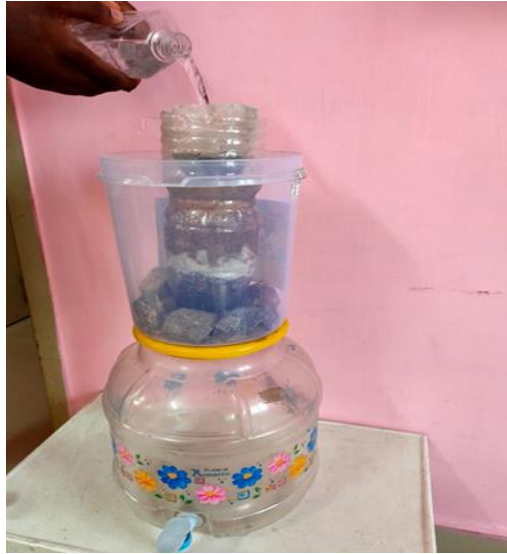
Fig: 4.27: Pouring of raw water for filtration
