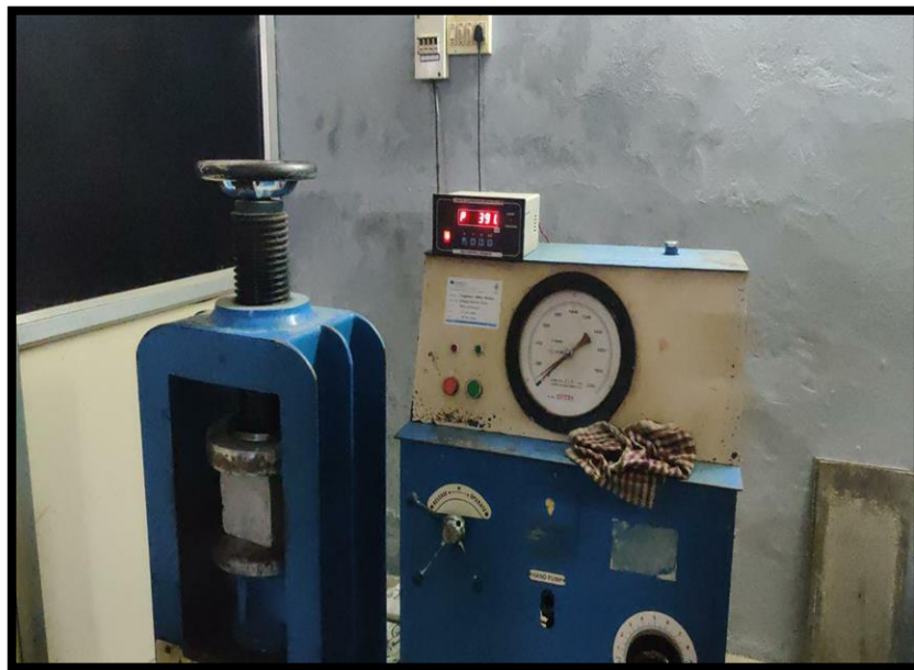
Fig4.1 Compression testing machine under load
