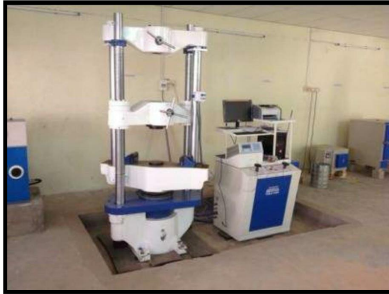
Fig.4.3 Flexural strength test Machine
