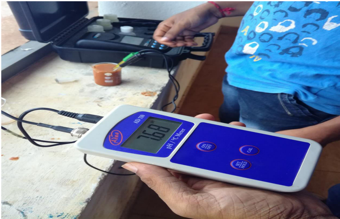
FIG4.1.5 WATER Ph TEST
