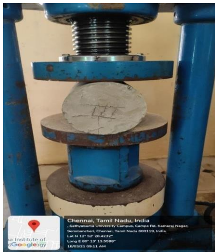
FIG: 4.18 Split Tensile Strength Test
