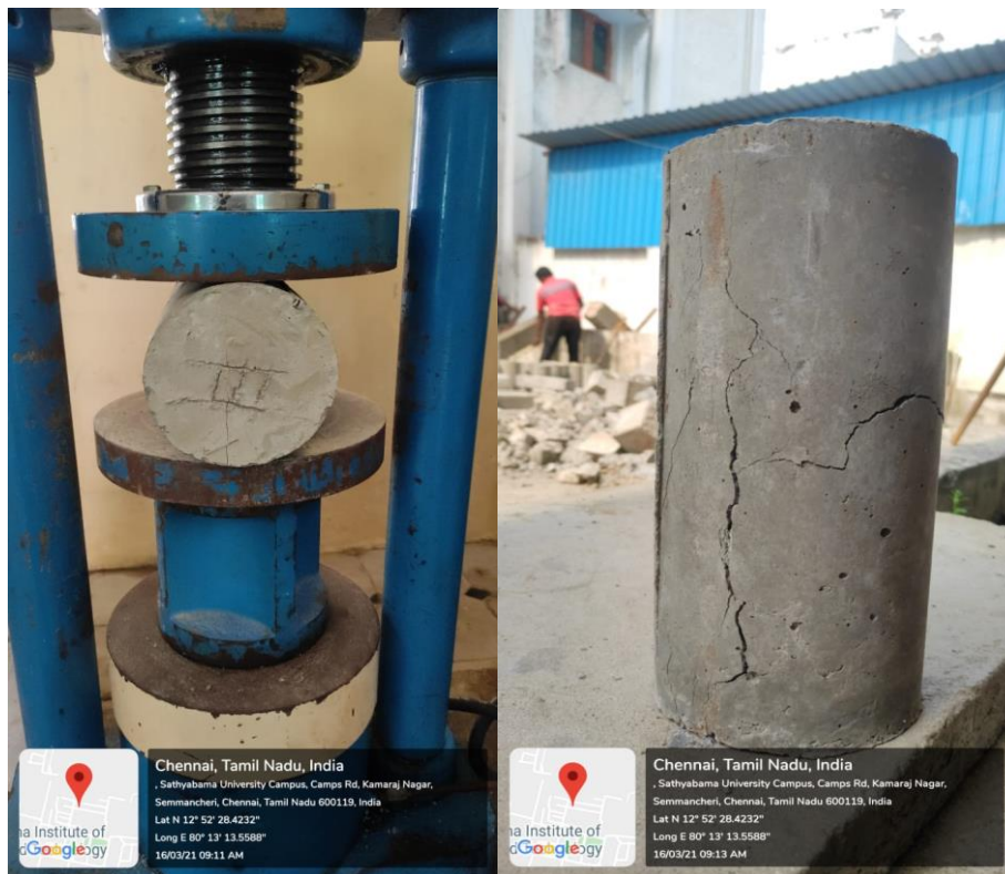
Fig 4.19 Split Tensile Test
