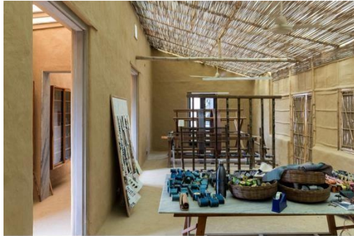
Designer's Studio, to create diffused light and semi transparent bamboo roof.
