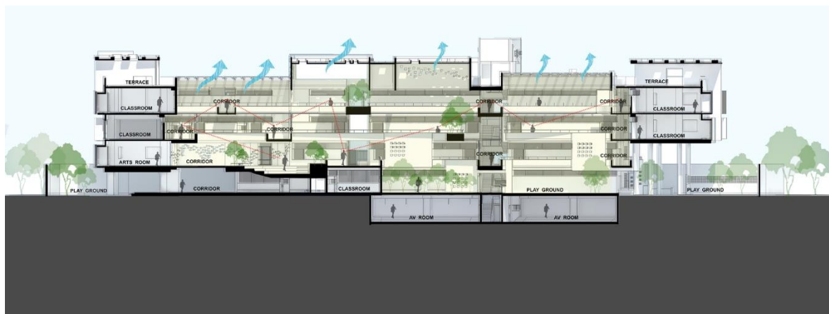
Fig 3.12 Section of the school with wind circulation
