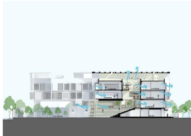
Fig3.11 Section with wind circulation
