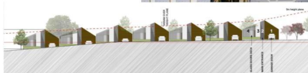
The roof apex was maintained at 5m above the ground
