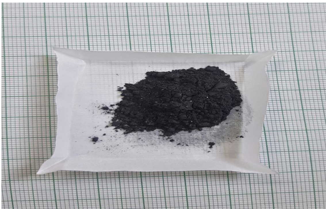
Fig.5.4 Final \text{SnTe}_{0.5}\text{Se}_{0.5} material after ball milling
