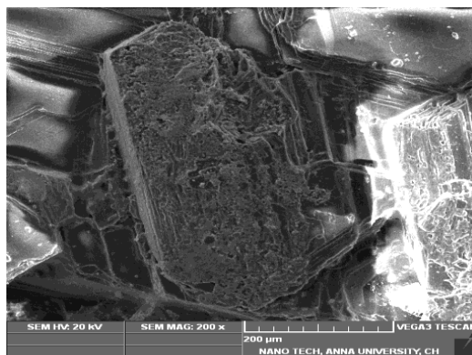
FIG 5.6 The surface morphology of Magnesium Cadmium Borate crystals
