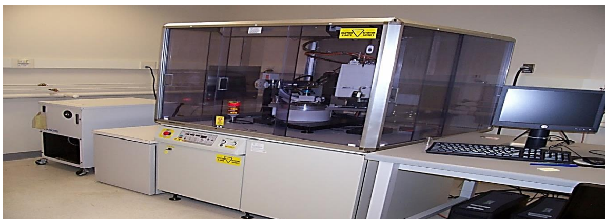
Fig 4.2 Instrumental setup of BRUKER Kappa Apex 2 CCD diffractometer
