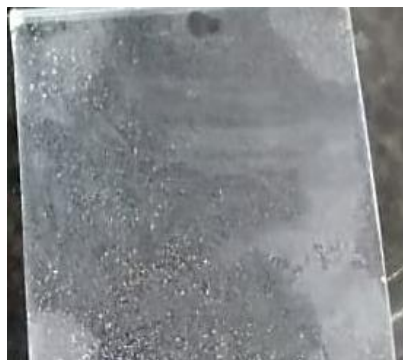
Figure.4.16 Pure SnO 2 thin film (100:0)
