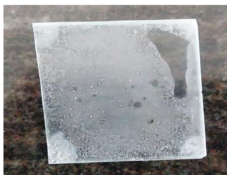
Fig.4.17 Fluorine doped SnO 2 thin film of doping ratio 90:10
