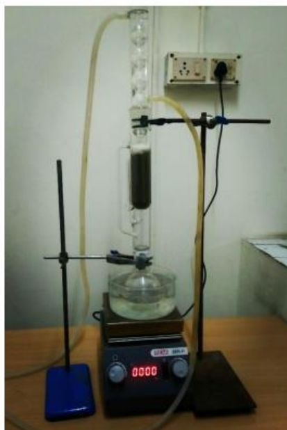
Fig.4.5. Soxhlet apparatus with the sample
