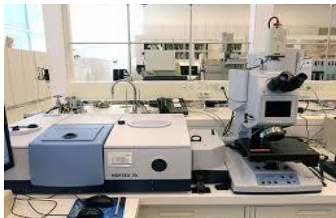
Fig 4.2 Fourier Transformer Infrared Spectrometer
