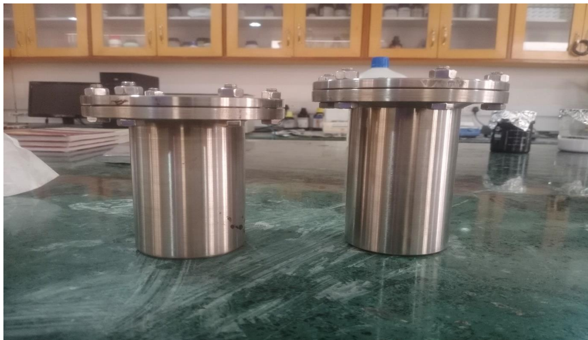
Figure 1.5.1.4: Hydrothermal method using autoclaves
