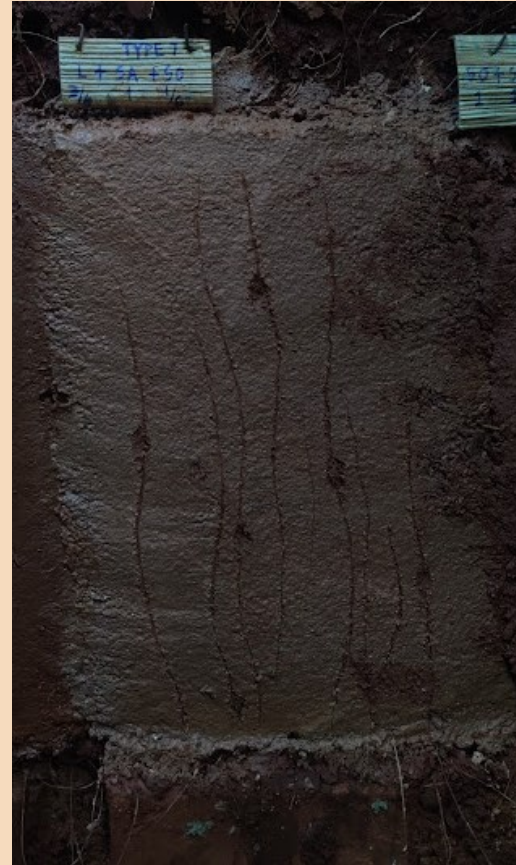
1soil+1sand+ \frac{1}{3} lime+ \frac{1}{4} rh+ \frac{1}{2} straw
