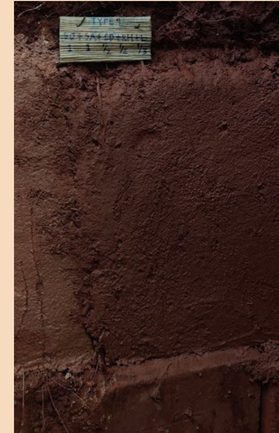
1soil+1sand+ \frac{1}{3} lime+ \frac{1}{2} rh+ \frac{1}{2} cd
