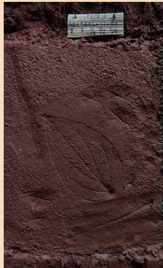
1soil+1sand+ \frac{1}{3} lime+ \frac{1}{4} rh+ \frac{1}{2} straw
