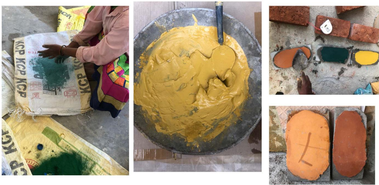
Mixing of oxide colour, white cement and grey cement.
