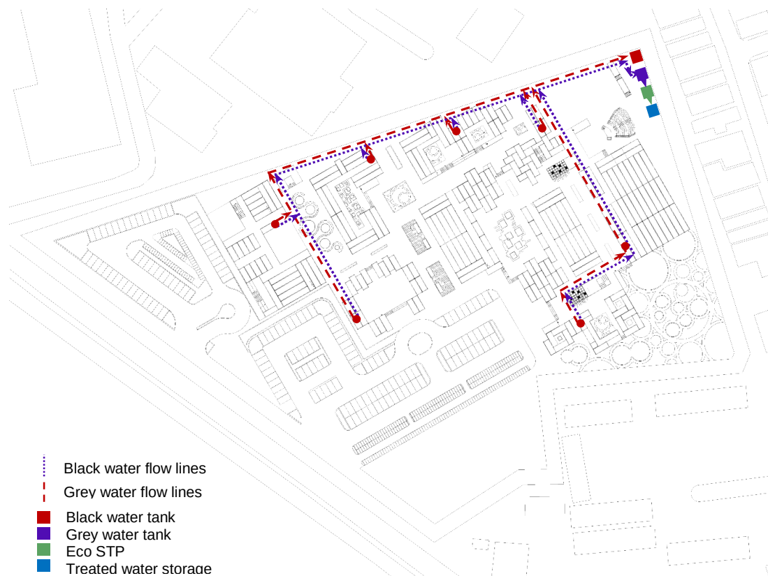
Fig 12.14 STP flow lines
