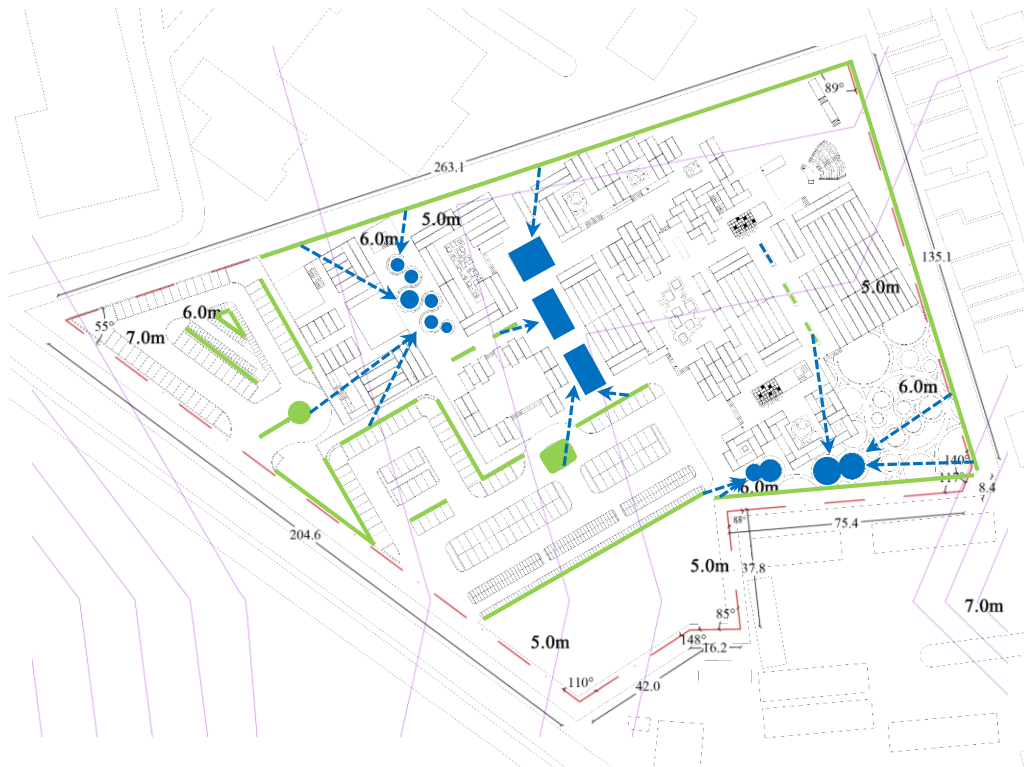
Fig 12.11 Bio swales RWH flow lines
