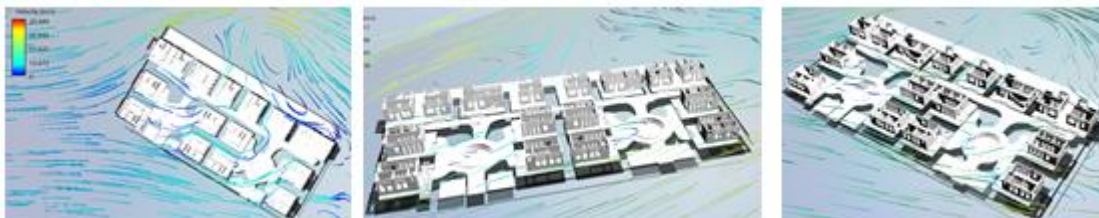
Fig 33 – Cluster model wind analysis, Ground floor
