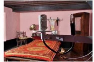
RH and temperature sensors in bedroom
