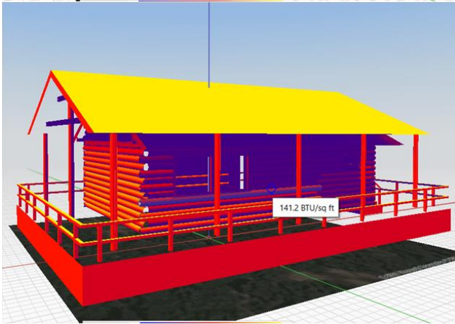
Fig 3.27 Solar radiation level in the month of July at 12 PM
