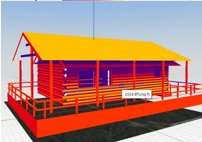
Fig 3.28 Solar radiation level in the month of January at 12 PM
