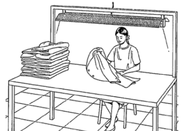
Figure 16: A bench light fitting for special workstations like quality control or packing tasks
