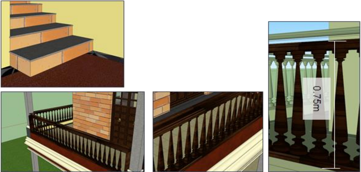
Fig 4.12.9: Staircase, railing and baluster details
