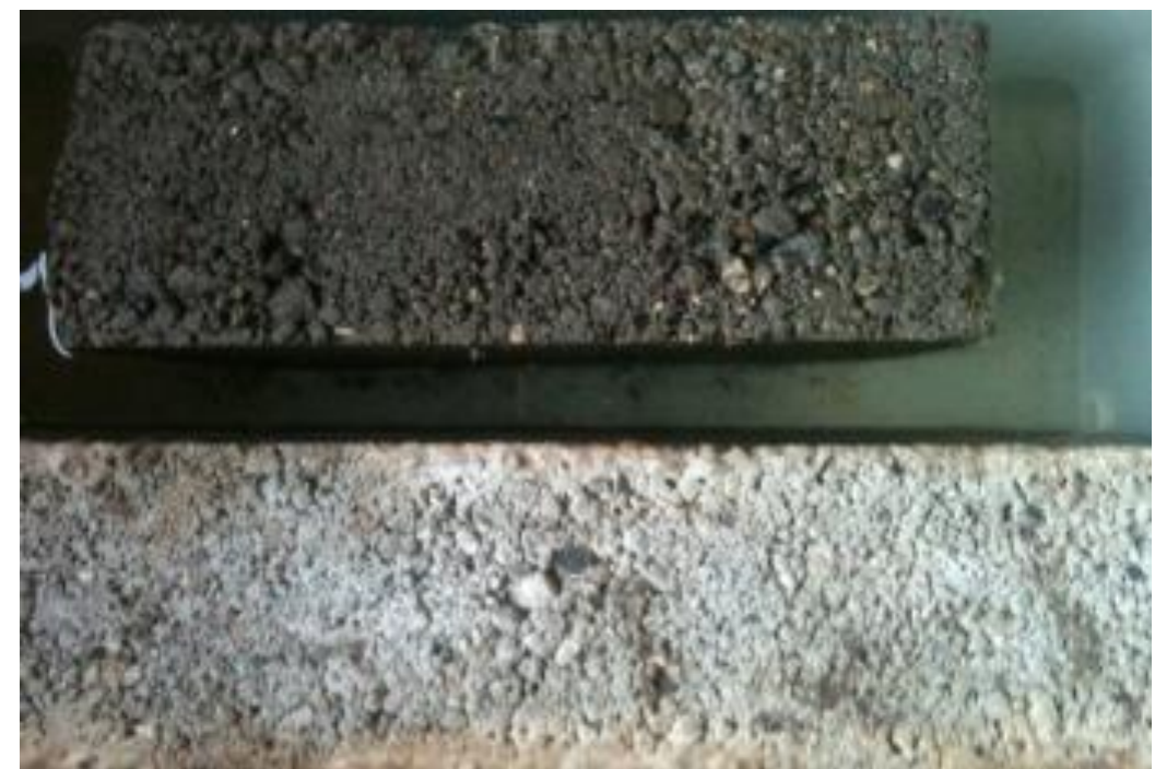
Comparing RADMYX untreated concrete (top) with a treated sample (bottom) in an immersion test
