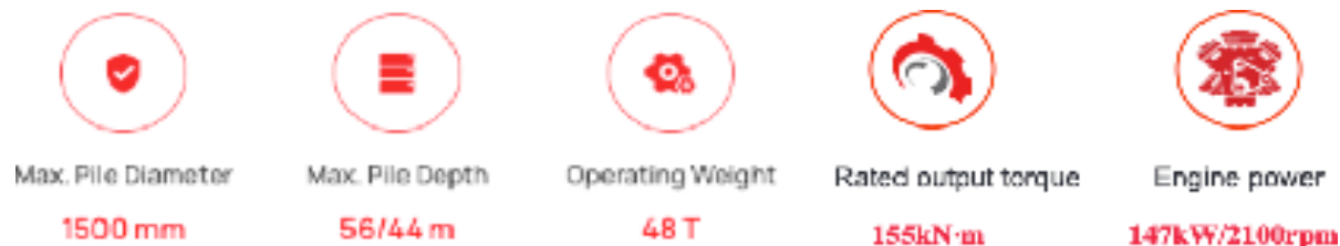
Figure 75 : Sany SR 155 - Main specification
