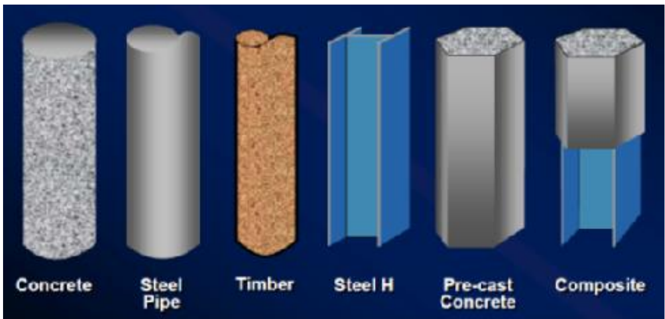
Figure 27 : Types of piles
