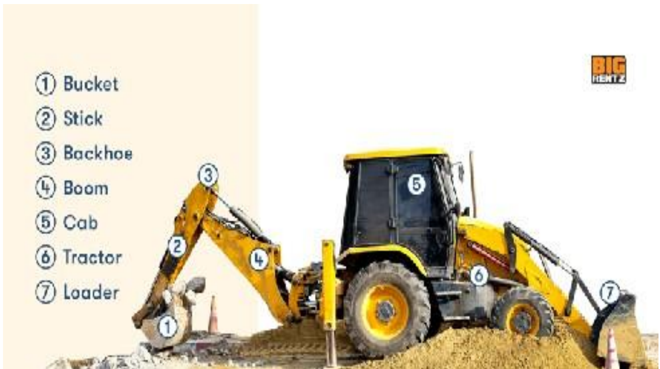
Figure 26 : Components of Backhoe Loader
