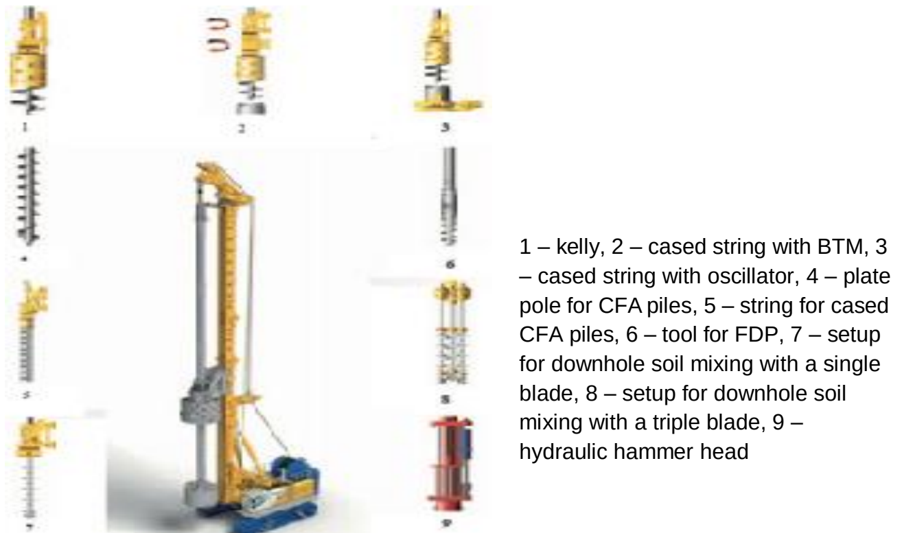
Figure 2: Components of pile driving machine
