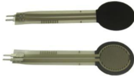
Figure 4.2 Front and back view of Force sensing Resistor
