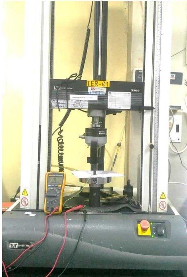
Figure 5.1 calibration of FSR sensors
