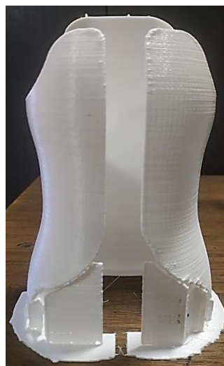
Figure 1.3 trial version of mini prototype 3d printed using PLA filament
