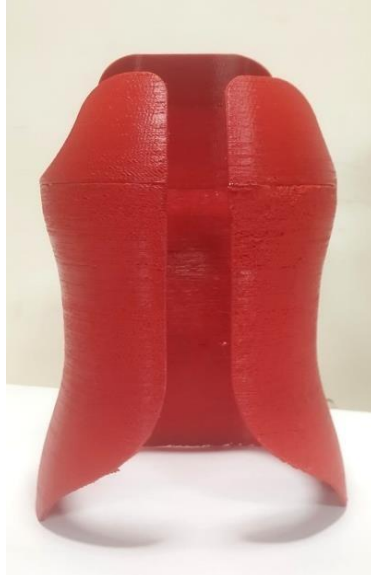
Figure 5.6 scoliotic brace fabricated using 3d printing technology
